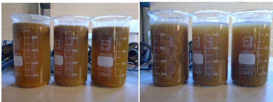
**Figure 2** Results of pH adjustment. From the left to the right pH: 5.5;6.0;6.5;7.0;7.5;8.0.
